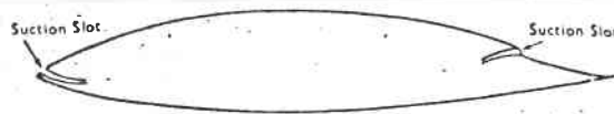
Fig. 16.—Shape of a suction aerofoil of the Lighthill type with two suction slots.
