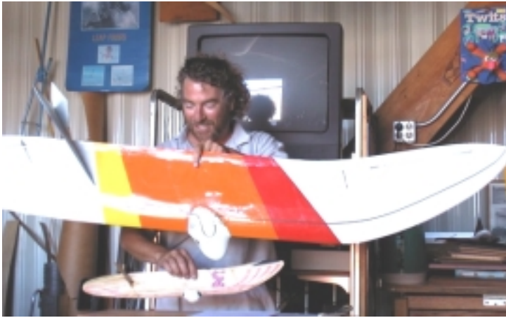
ABOVE: Dave holding his early hand launch test model (bottom) and the first R/C oblique wing. You can determine the flight sweep by looking at the vertical fin position and, the different configuration of the left (leading) wing tip.
