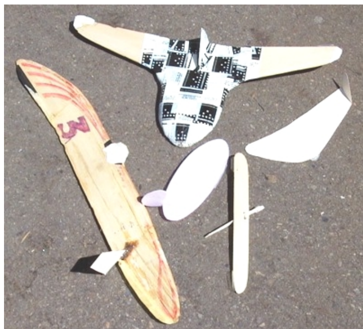
ABOVE: Clockwise from left: initial concept test model; blended wing test model of current project; maple leaf test model; early test model with a fuselage section, and; (center) a small foam oblique toy wing designed and produce by Les King.
