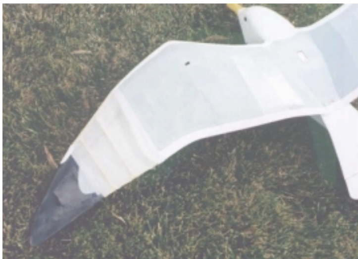
ABOVE: The Seagull model has been equipped with a flexible section of wing to allow for a smoother flow transition for the tip-aileron. The wing section is covered with ripstop nylon (from an old parachute)
