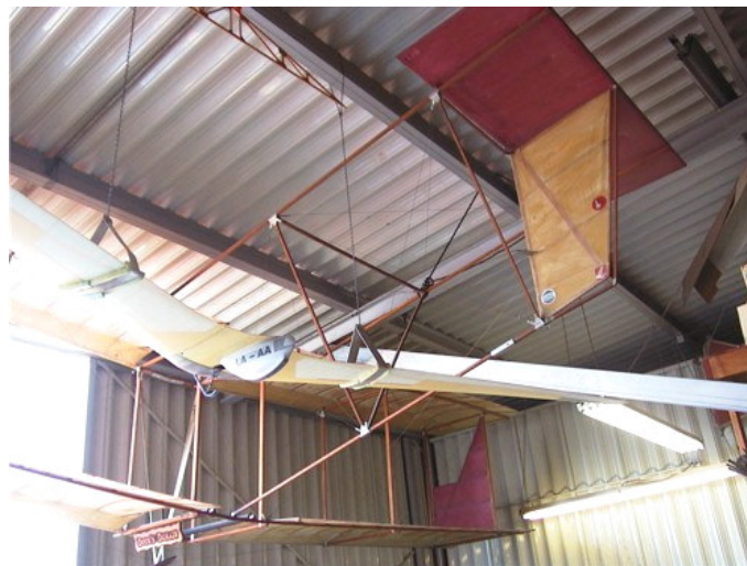
ABOVE: From this view of the Horten you can also see the framework of the Waterman glider. The middle triangular bay in the tail boom was added after the spin accident to provide additional strength and stability to this section of the structure.
