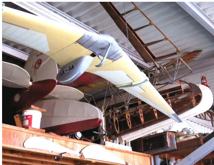
ABOVE: More of the Horten IV with the Robin wings (dark wood) and Super Bowlus wings (white). This is also a good shot of the Gottingen airfoils.
