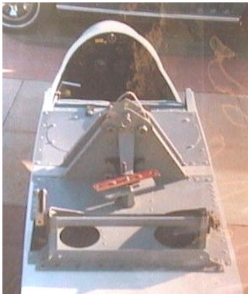
ABOVE: This is a shot of the carry through section of the fuselage showing the flap torque tube at the bottom.
