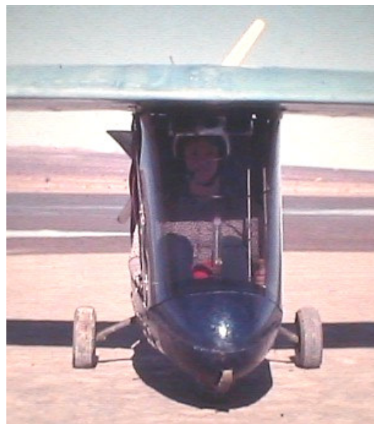
ABOVE: This is a front view with the nosewheel retracted in what can be used as the landing position. It actually makes the plane look much sleeker.
