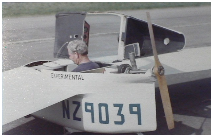
ABOVE: 12 hp engine with homemade belt drive in the Motor Floater.
