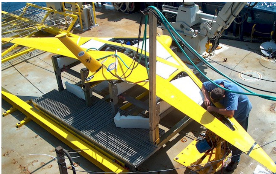
ABOVE: The current XRay version sitting on the mother ship launch pad. Note the lack of winglets, addition of the communications vertical that can partially fold down for transport and, the larger nose cone area.
