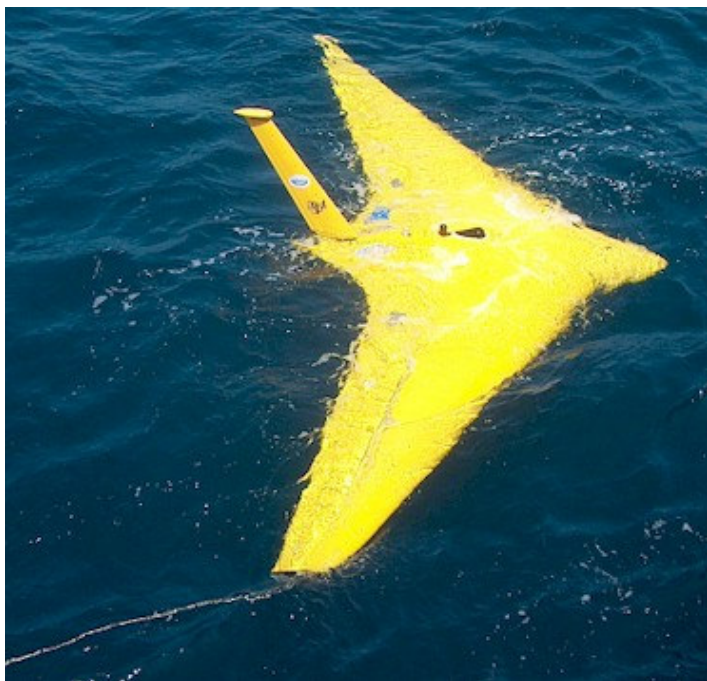
ABOVE: XRay on the surface with the right tip deployed to extend the retrieval line.
