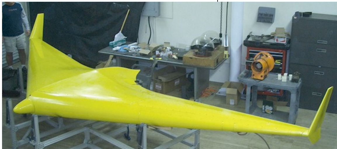
ABOVE: Stingray version of the underwater glider. Note the use winglets and the smaller size of the nose cone when compared to the subsequent XRay glider.
