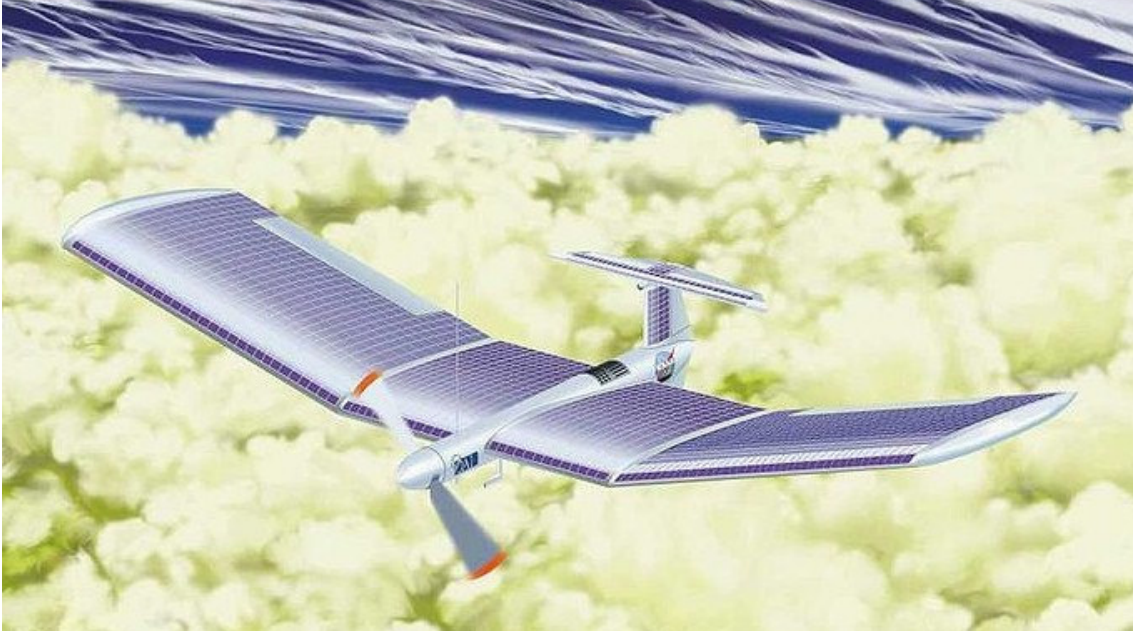
Concept for a solar-powered aircraft to explore the atmosphere of Venus. Image by Les Bossinas, NASA Glenn Research Center. See Geoffrey A. Landis, Anthony Colozza, and Christopher M. LaMarre, Atmospheric Flight on Venus , AIAA 40th Aerospace Sciences Meeting and Exhibit, American Institute of Aeronautics and Astronautics, Reno, Nevada, January 14-17, 2002. http://gltrs.grc.nasa.gov/citations/all/tm-2002-211467.html
