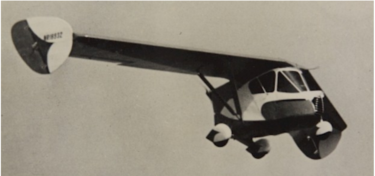
Waldo Waterman's Arrowbile flying car. The idea behind the Arrowbile was to develop a transmission drive system that could operate the propeller for flight and the rear wheels for ground operation. His flying car can be seen at the Smithsonian National Air and Space Museum. Source: http://thefrontblog.wordpress.com/tag/paducah/
