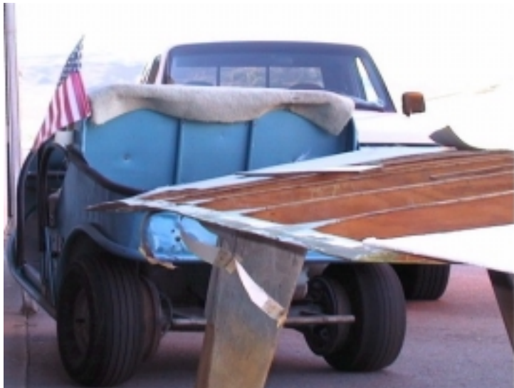
ABOVE: You can see from this angle how the Rigid Midget's trailing edge has an upward curve on the inboard section. You can also see that the ribs are solid wood, to which the comment was made that the glider couldn't be flown in lightening conditions since there were no lightening holes in the ribs.
