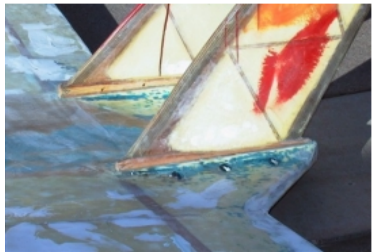
ABOVE: This is the vertical attachment point. It sits in a box and is held in by 3 aircraft quality bolts going through the box and base of the fin.
