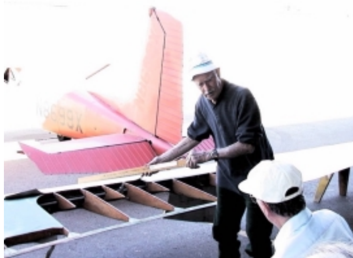
ABOVE: Here you can get a good look at the rib placement and what is causing the curve in the trailing edge. Since they are mounted at this angle on the spar, they would have to be removed to correct the condition. The short ribs in between the longer ones only serve to smooth out the fabric coming off the D-tube section.
