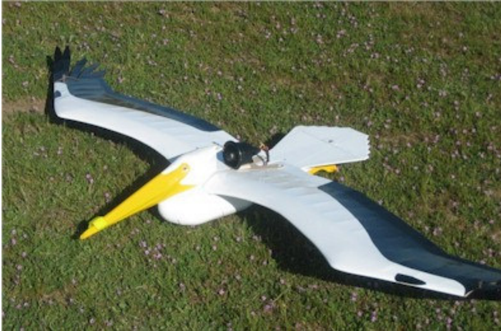
This is Bob's White Pelican with the electric fanjet power pack for longer flights. These small fanjets are a perfect match for this type of application with Bob also putting one on his Raven model.
