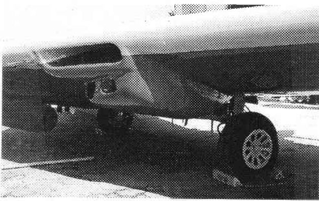
ABOVE: The left main gear using a P-51 wheel assembly, and the air intake for the Franklin experimental engine.
