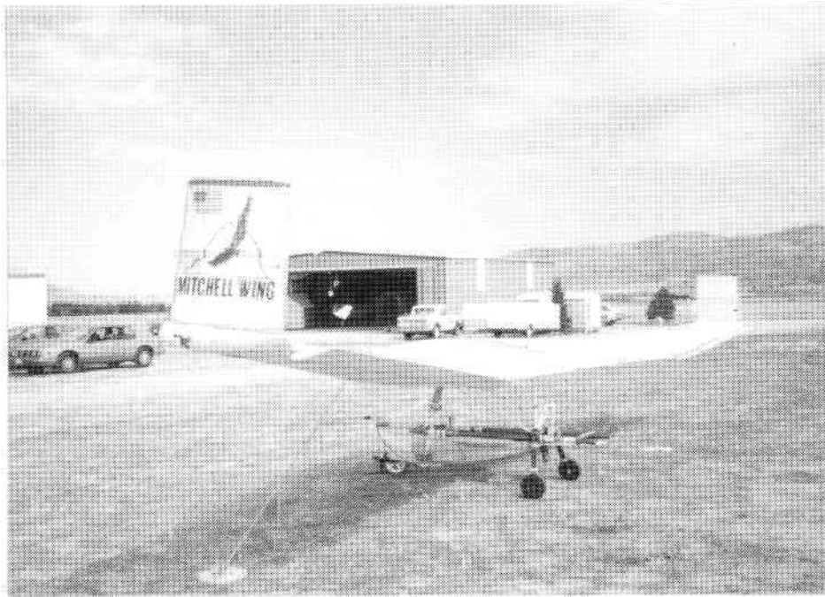
ABOVE: Chuck Rhodes Mitchell Wing formerly owned by George Worthington. Note the modified pilot's cage with the single nose wheel and dual rear wheels which make landings much easier in no wind conditions. Photo by Andy Kecskes.
