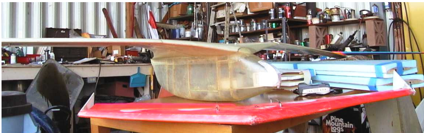
ABOVE: A view of the fuselage pod and the gull shape of the center section. The red glider in front is the Zagi they used for initial testing of some ideas.
