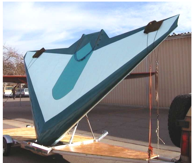
ABOVE: Top view of Gerry's Skyler. It still needs the tow attachment harness and small windscreen just behind the dark Vee at the front. BELOW: The underside showing there is a slight step to help it break the water.
