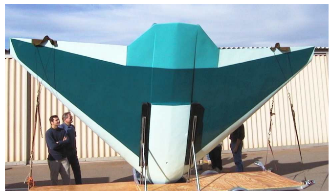
ABOVE: Top view of Gerry's Skyler. It still needs the tow attachment harness and small windscreen just behind the dark Vee at the front. BELOW: The underside showing there is a slight step to help it break the water.
