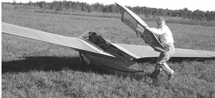
ABOVE: The top hatch being placed on the Horten IV before a test flight.
