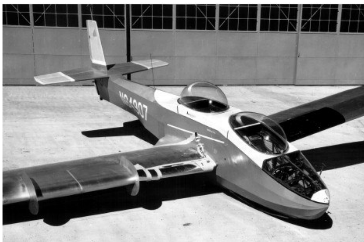
ABOVE: Here is a shot of the boundary layer control TG-3 where you can see the heavily modified right wing and extensive conversion into a flat top configuration.
