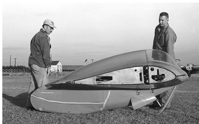
ABOVE: The Horten IV center section before the wings were attached. Desz Georges-Falvy is at the right.
