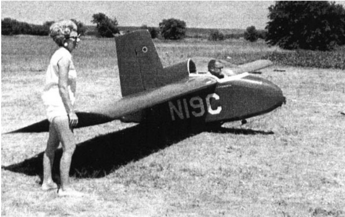
Central fin version of EPB1-C. http://www.nurflugel.com/Nurflugel/Fauvel/plank_3.jpg
