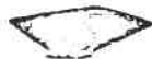
AERODYNAMIC DINNER-PLATE.— This is the Canova Rhomboidal Wing, built and flown in Italy during 1935. The pilot sat on a skid slung under the wing, which had a fin and rudder attached to the upper surface; elevators and ailerons were provided. The aspect ratio was about 2. Stability longitudinally was satisfactory but laterally was deficient.
