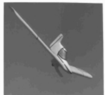
REVISED VERSION SPAN = 36 FT. LENGTH = 8.33 FT. HT = 5.4 FT AREA = 93 SQ. FT. WING JOINTS 8 FT OUT TAPERED OUTER PANELS ZERO TWIST INBD CHORD = 3 FT. OUTBD. AVE = 2.25 FT ASPECT RATIO = 14 SWEEPBACK = 13° AIRFOIL = 63 515 REFLEXED 0 DIHEDRAL OUTBOARD DIFFERENTIAL ELEVONS FOR PITCH AND ROLL CONTROL CENTERLINE FIN- DIRECTIONAL STAB. ELEVON INSET SPOILERS-DIR CONTROL 154 # EMPTY WT. 154 # P.L. 308 # GROSS WT. WING LOADING = 3.3 P.S.F. GROSS WEIGHT / SPAN SQUARED = 0.24
