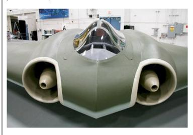
The big mystery was whether this was a stealth aircraft developed more than three decades before modern stealth technology emerged. Could the wedge-shaped jet almost completely formed from wood actually evade radar detection of the time. This made military analysts wonder if the outcome of the war would have been different had the German's introduced this fighter in any great numbers during the war.
