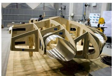
**Above:** This is the center section during the buildup phase. The original had a steel tube inner structure so special paints were used to simulate the effect it would have on the radar signature.
