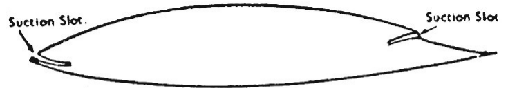
Fig. 16.—Shape of a suction aerofoil of the Lighthill type with two suction slots.
