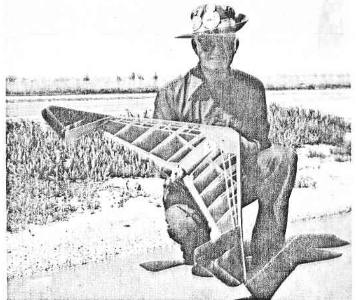
Very successful tailless design by Tex Rickard from 1938 Frank Zaic year book. This ship is powered by Cox .049 and flown in 1/2A Texaco.
