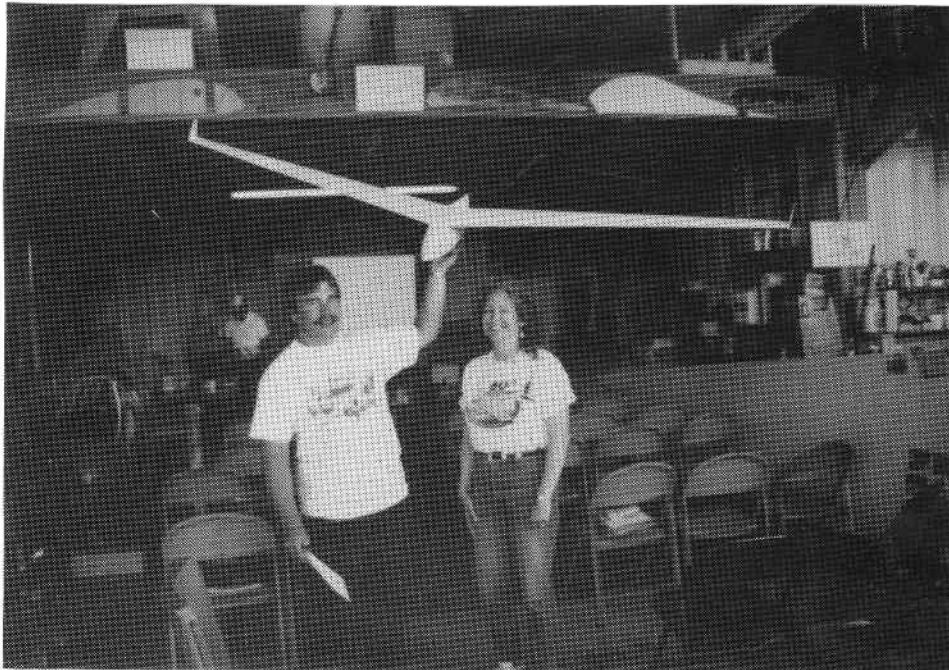
ABOVE: Craig and Nancy Roberts showing off Craig's concept model of his joint project with Floyd Fronius. The full scale version will be 15 meters with elevons and drag rudders.
