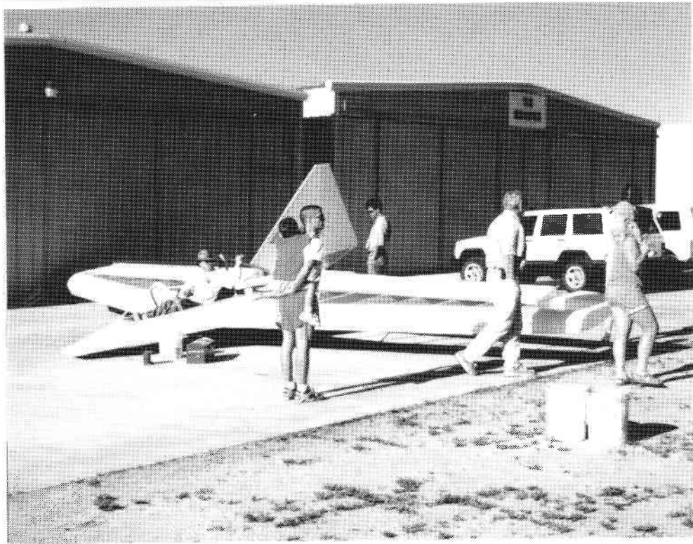
ABOVE: Front view of Les King's The Primer as seen at the Vintage Sailplane Association meet at Tehachapi, CA. The extensive use of foam can be seen as well as the strake type nose extension.
