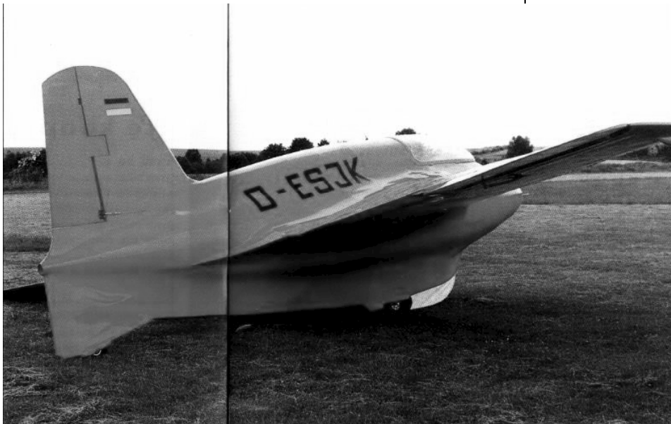
ABOVE: Josef Kurz's replica glider. Note the faired tail wheel and main gear tire which are obviously not quite like the original. Also note the more conventional style glider skid versus the retractable landing skid of the real Me 163.
