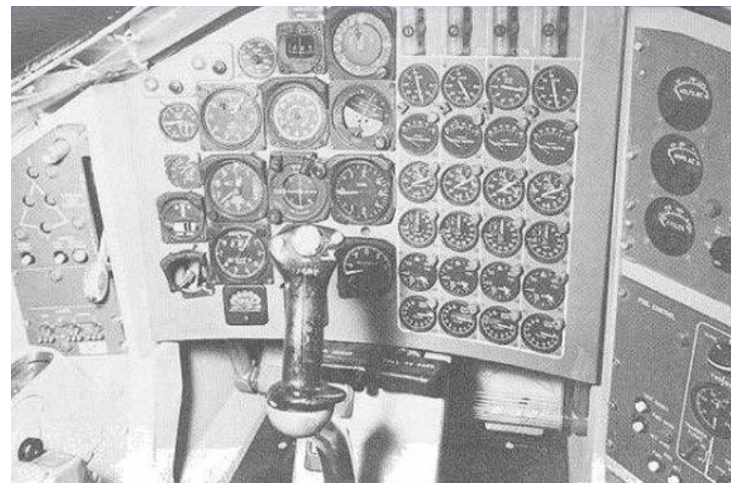
The pilot's main instrument panel for prototype aircraft 55-660. With the exception of the Mach meter, the instrumentation was conventional for a multi-engine aircraft.
