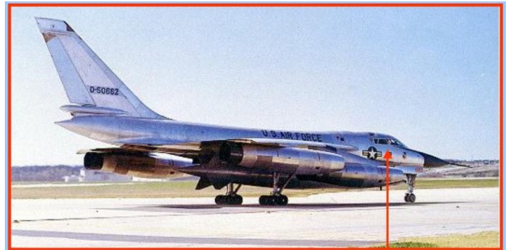
A TB-58 taxiing for takeoff. Note the extra windows. The TB-58 has no navigator. He is replaced by an Instructor Pilot who sits behind and offset from the Pilot. No capsules are on the TB, only the original ejection seats.
