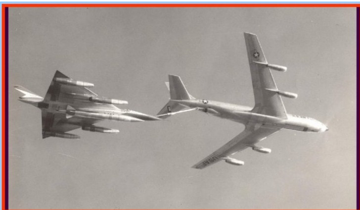
Pulling into the contact position to air refuel with a KC-135 tanker aircraft
