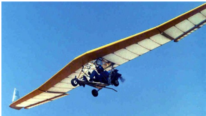
ABOVE & RIGHT: These are not Dale's ship, but reminds everyone of the basic layout of the Mitchell B-10 wing.
