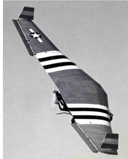
ABOVE: This shows the location of the wing tip rudders so you can see how they are in-board of the tip and relatively large.
