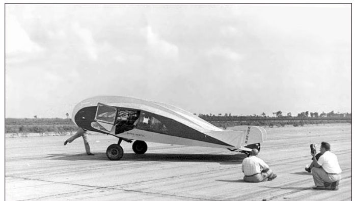
ABOVE: Original Horton prototype (before the one shown in last month's newsletter and promotional videos) during initial testing. Entry door can be seen in end-plate, with the pilot sitting in the middle of the wing. Source: Al Backstrom.
