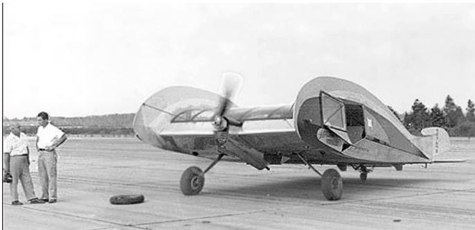
ABOVE: Original Horton prototype during an engine runup test. Notice no "airbrakes" as in the later model. Source: Al Backstrom.
