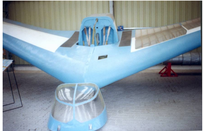
ABOVE: IA-41 URUBU (Ho-XVc) was a side by side glider, built in 1951 in Argentina. It was the first glider to go across the Cordellera de los Andes, piloted by Heinz Scheidhauer. Central section is made of wood and steel tubing (notice waling strips). Part of the story of the Horten flying wings in Argentina is documented in the book "Las Alas de Peron" (Peron's Wings) by Ricardo Burzaco published in Argentina (1995) ISBN 987-95666.
