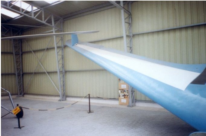
ABOVE: Starboard wing showing small all movable rudder that replaced the original spoilers, which were hated by some glider pilots. The sky-blue leading edge portion corresponds to the wooden torsion box; behind it, all is fabric. Over the rudder it can be seen an Avro-La Clerva rotor blade.
