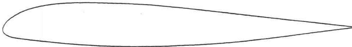
Airfoil used on Marke Pioneer has less reflex
