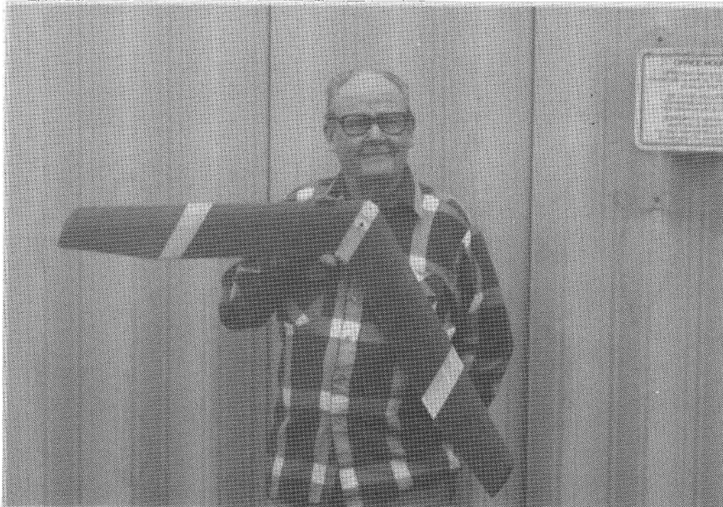
ABOVE: Alfred Faulkner holding his contest winning flying wing model of his own design which is now 9 years old. It has a 40" span, 30° sweep, washout at the tips, flat bottom airfoil, and maximum thickness in the forward portion of the airfoil. Photo by Bob Fronius.
