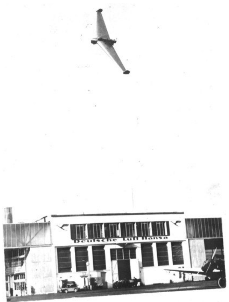
ABOVE: Gronhoff sweeps low over Tempelhof Airport (Berlin), with the Delta I on October 25, 1931, while on a test flight of the aircraft for Lippisch. Unfortunately, airport officials who gathered to watch were alarmed and demanded that a tailplane be added before a certificate of airworthiness could be issued. (From Unconventional Aircraft “The notable design detail of the Delta I was that while the leading edge of the wing was still swept back at a comparatively shallow angle, the sweep of the trailing edge was eliminated by having it run a straight line from tip to tip. This is historically significant in that it started the development of the delta wing, which was not to become successful until after World War II – and then proved to be pioneered by Lippisch.
