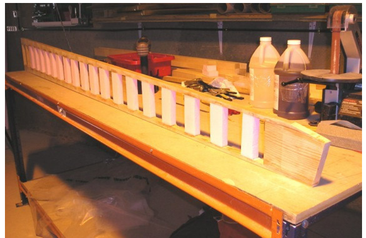
ABOVE: This is the outer wing spar on the jig table.
