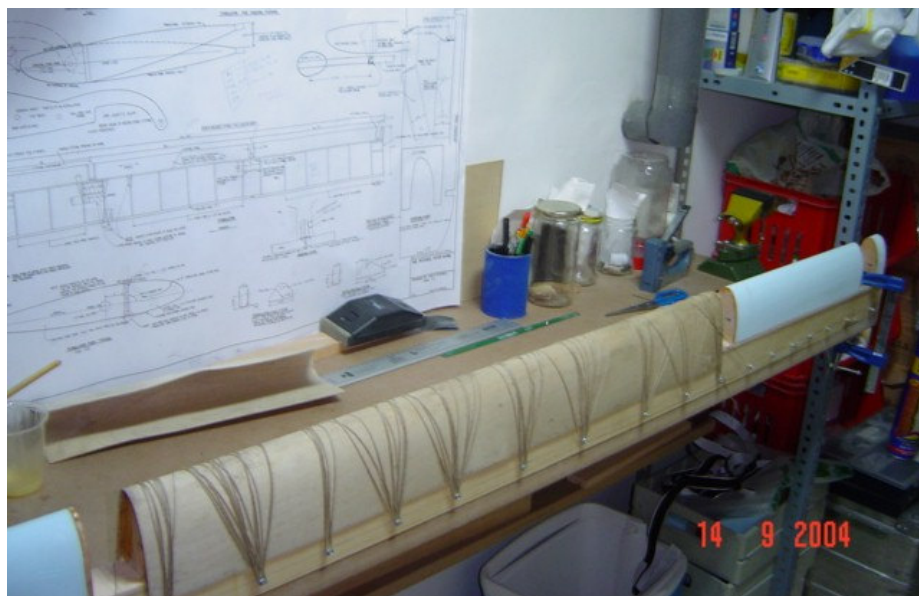
ABOVE/BELOW: This is the stabilator in Adolfo's jig. This looks a lot easier than using a lot of sand bags to hold everything in place while it dries.
