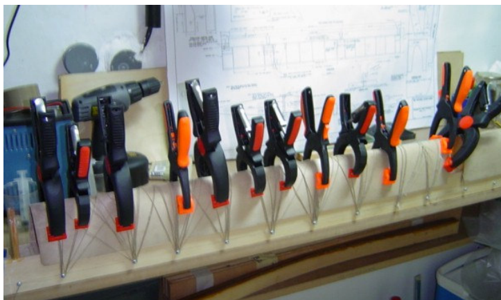
ABOVE/BELOW: This is the stabilator in Adolfo's jig. This looks a lot easier than using a lot of sand bags to hold everything in place while it dries.
