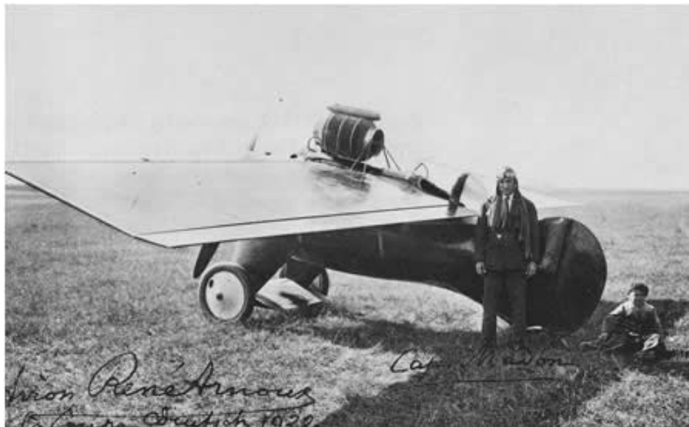
French ace George Mix Madon, who had 41 dogfight victories in World War I, poses by the futuristic Simplex Arnoux racer of 1922. The pilot's vision forward and down was severely restricted by the Lamblin radiator perched on top of the fuselage and the expanse of the Arnoux "flying plank" Wing. Speed was 236 mph. Source: http://www.century-of-flight.net/Aviation%20history/flying%20wings/europe_interwar.htm
