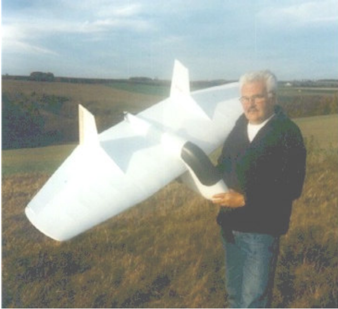
ABOVE: Early scale model being held by an unknown individual. Note the difference in the rudders between this model and the final prototype. The model has full height vertical stabilizers with rudders versus the version seen on page 4. (Photo courtesy of Koen Van De Kerckhove)
