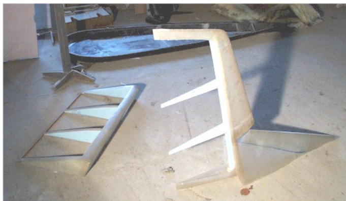
ABOVE: Rudder being assembled. Note the small fin area at the right edged of the vertical portion of the rudder. (Photo courtesy of Koen Van De Kerckhove)
