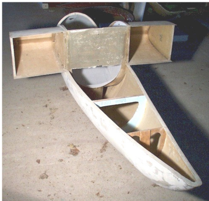
ABOVE: Here is a shot of the fuselage from the rear looking at the center section spar area. (Photo courtesy of Koen Van De Kerckhove)
