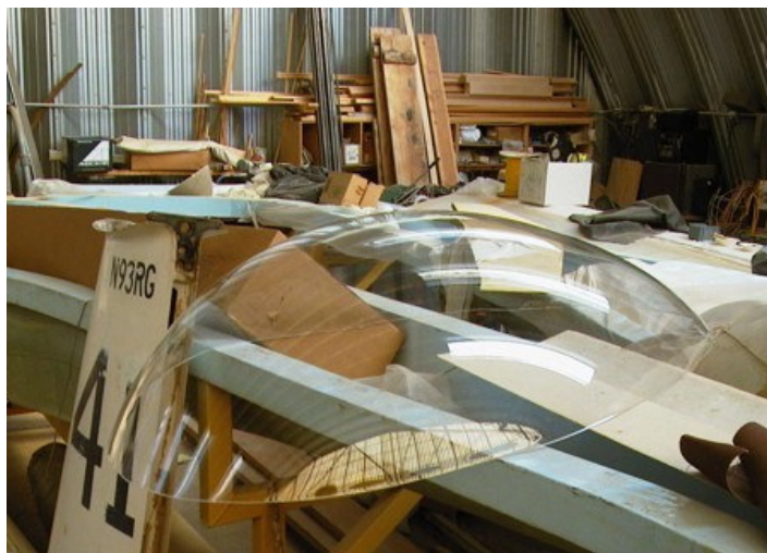
Here is the almost finished product. George has taken it out of the frame and trimmed off the flange. The canopy is flexible enough to reshape it to several different frames so it can be adapted to various sailplanes. You can get an idea just how clear and undistorted it is.
