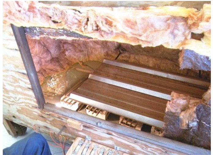
This is a shot of the heat box's interior. On the bottom you can see the 4000 watt heaters underneath a diffuser panel. You can also see the fiberglass lining and a portion of the switching panel. I imagine that when all the heaters are operating the electric meter is spinning probably to the point of seeing the needles moving on the indicators.
