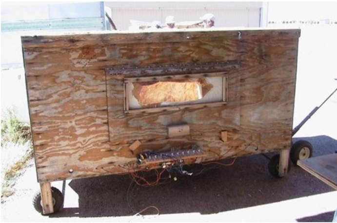
This is the heating box that George built. It is fully mobile with steerable wheels at the right end. The window allows viewing the glass while it is heating up without letting the heat escape. The switches below the window control the heaters (simple on/off) mounted in the bottom. The whole unit is simple and very functional as you will see from the finished product.
