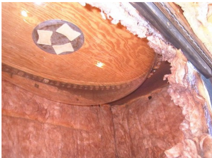
Here is a shot of the almost finished canopy hanging from the form. Now you can see why all the clamps are necessary. Even in this state you can see the glass is very good optically, partially due to the glass quality and partly because of the very slow expansion that allows the glass to maintain a consistent thickness.
