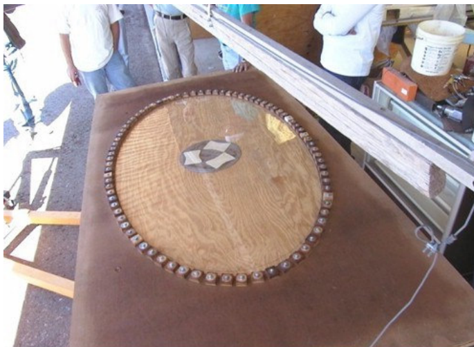
Here you see the lucite glass mounted on the forming board. It takes all those clamping pieces to properly secure the glass so the edge won't move during the expansion process. The area in the middle is where the air pressure fitting will be installed from the back side. Note the loop on the cable in the right foreground. It comes into play after flipping this whole piece over using the hoist.
