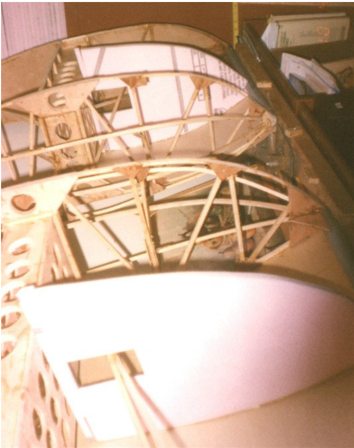
Here is a shot of what appears to be the two wing tip sections set side-by-side. Obviously he has put a lot of work into building the ribs and spar section trying to keep them as light as possible.
