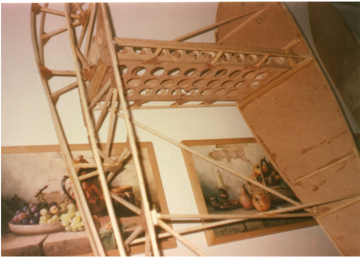
This is a shot of the full size wing tip section. The full faced rib on the right is the inboard end, and the left side is the structure for the formation of the tip shape. Based on this picture, it can be assumed that the tip would be covered with fabric to achieve the desired shape.
