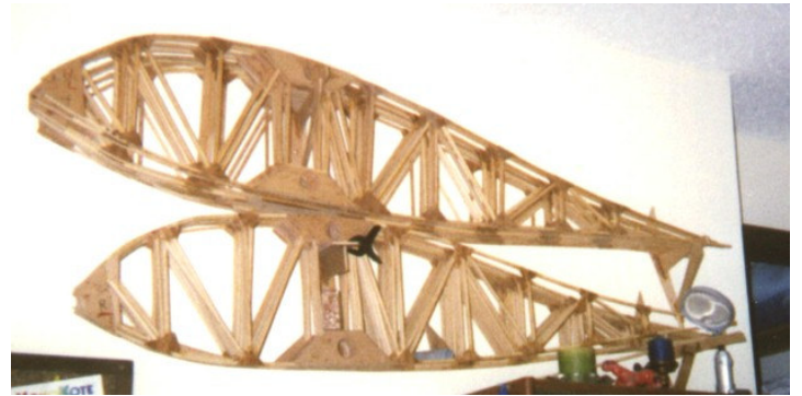
This shot was labeled as being 18 ribs, obviously hanging from one of the apartment walls. You can see the reflex in the airfoil in this view.
