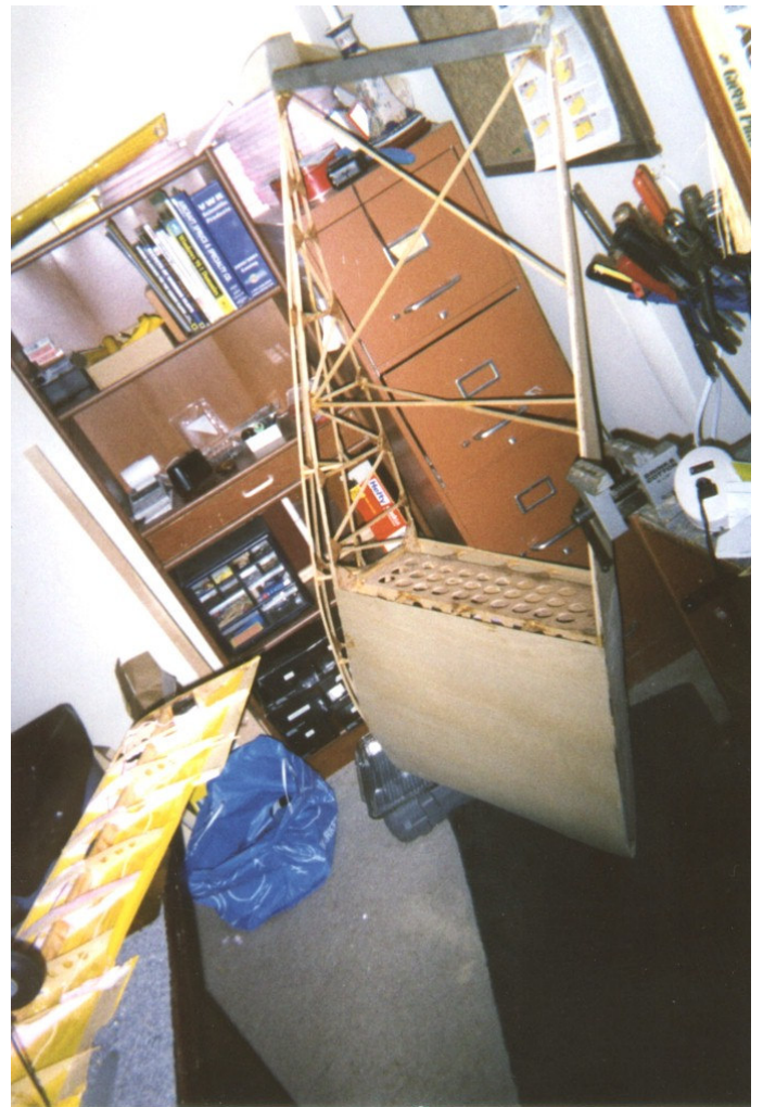
This shows both the model's underside uncovered and one of the wing tip sections with part of the D-tube sheeted back to the spar. It also gives you an idea of the limited amount of space Joe was utilizing in putting together his dream wing.
