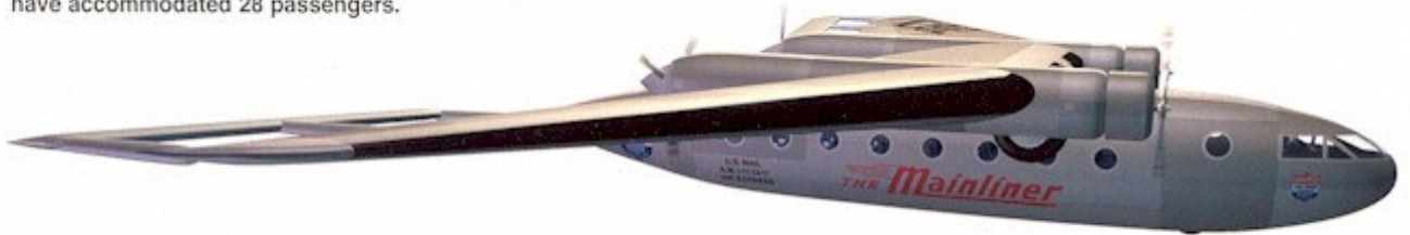
Side view of the Boeing's beautifully streamlined and unorthodox airliner study. The cigar-like fuselage would have accommodated 28 passengers.
