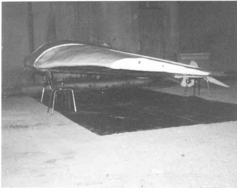
A side view of Alain Mirouze's low aspect ratio hangglider. Note that there are no tips in this view, but the in-flight shot on tow clearly shows the addition of tips.
