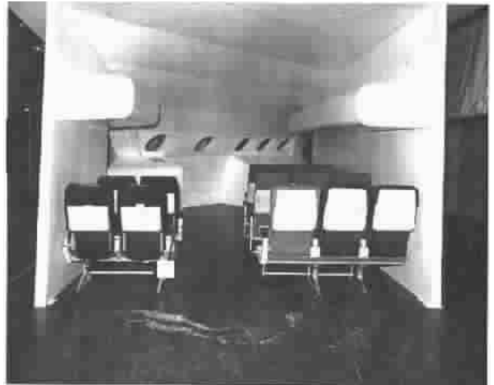
ABOVE: Typical passenger section looking toward the leading edge. Note the heavy vertical bulkheads needed to support pressurization loads.
