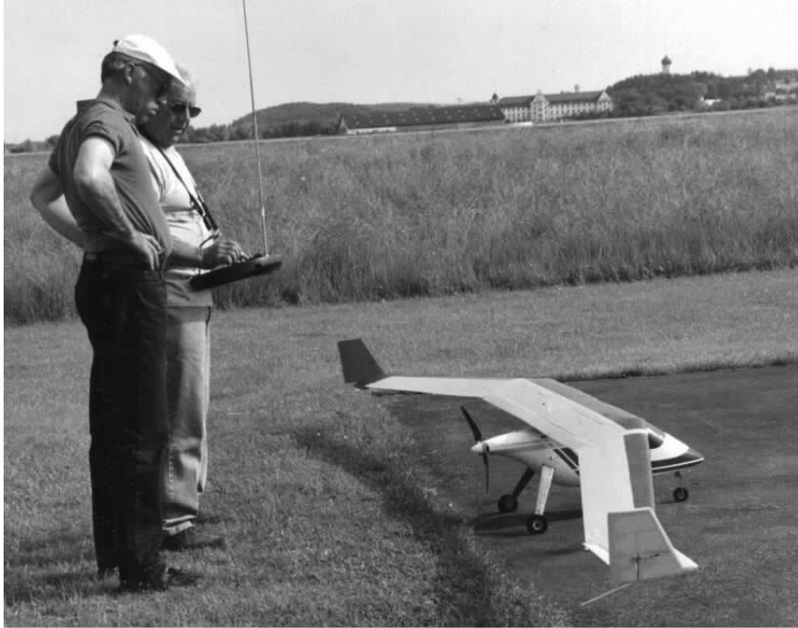
Thomas Bircher (at the controls) and friend getting ready for a flight of the LEA 23. This version features a pusher propeller, but based on recent questions it appears they may be headed for a jet powered version in the future. (ed. We hope to have more on this next month.)
