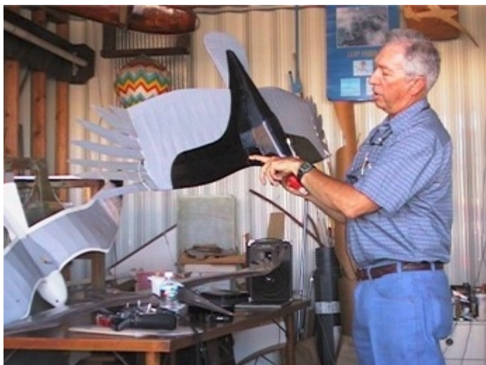
ABOVE: Bob is showing us where the aileron servo is now located driving a carbon rod out to the tip feathers. BELOW: You can see the feather angles, especially those at the leading edge from this shot.
