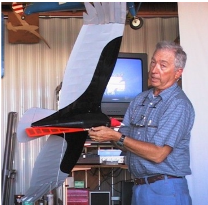
ABOVE: Bob is demonstrating the detachable stability fin now being used to high start the models, in this case the Turkey Vulture. The fin is actually slipped into a slot in the belly.
