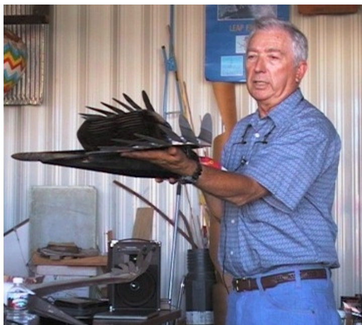
ABOVE: You can see the negative angle on the left wing tip in this shot and how it puts twist into the wing. You can also see the slight "V" shape of the horizontal tail and elevator. BELOW: Here is the Seagull in flight, with the radio antenna trailing. Photo courtesy of Bob Hoey.
