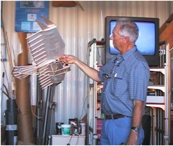
ABOVE: Bob holding the Leonardi de Vinci concept model. You can see the tip aileron configuration and that the aft portion of the wing is a single flat surface. You can also see that the ailerons are in a positive position which is not a normal flight position. BELOW: You can see the planform of this design.
