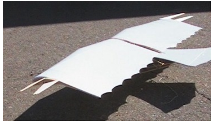
ABOVE: Here you can see the left aileron in a more normal flight position. You can also see the slight up on the elevator giving you an idea of its size.
