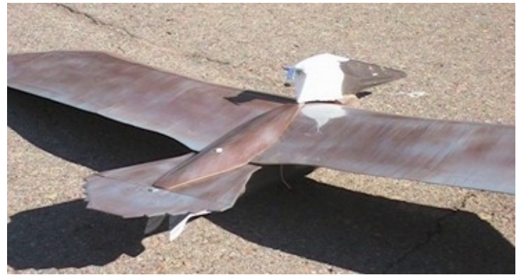
ABOVE: Here you can see the "feet" that were added to provide some additional stability. BELOW: Another shot of the tip feathers showing the upward curvature and the flatness of the aft feathers.
