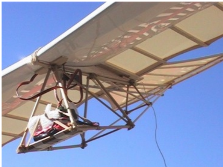
ABOVE: Here is a good look at the pilot cage and some of the wing structure. The radio gear was supposed to be placed inside of "Ken" the pilot, but that is another story.
