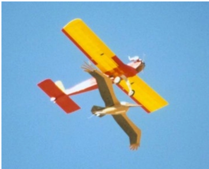
ABOVE: Here is the Pelican being launched from the mother ship. This is how a majority of the test flights began. The landing gear on the plane was extended several times to make room for the particular glider being launched. Photo courtesy of Bob Hoey.
