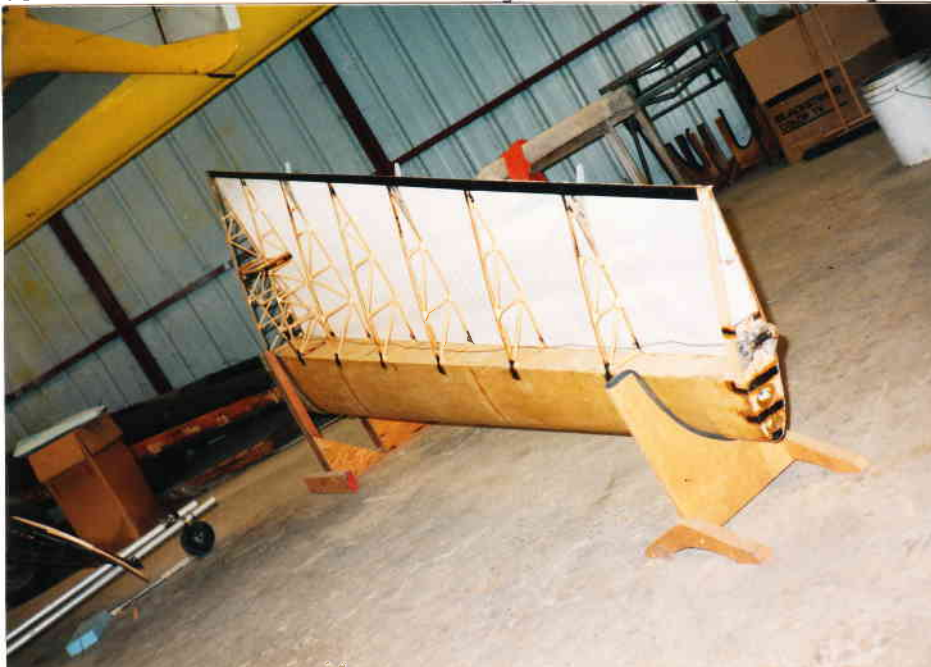
ABOVE: Left outer wing panel looking at the tip end with tube for mounting tip rudder. The three protrusions from trailing edge are hinge points for stabilator.
