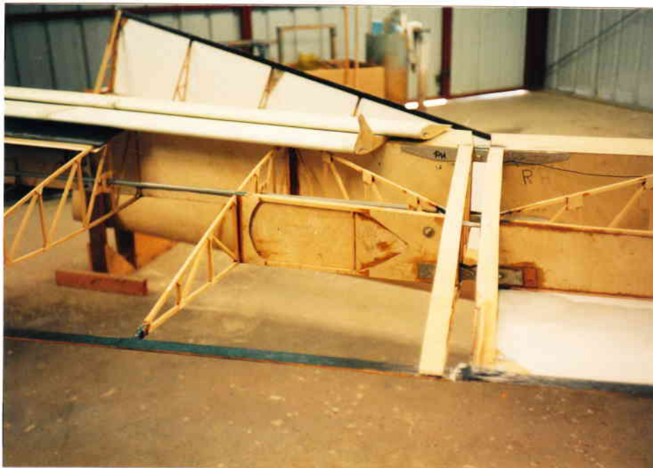
ABOVE: Right wing outer panel joint showing rear sub-spar and fittings. Stabilators (elevons) laying on top of wing.
