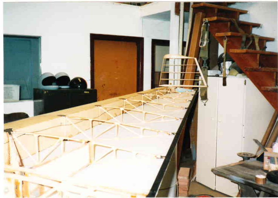
ABOVE: Right outer panel looking from the center section joint. Tip rudders move outboard only, and be move simultaneously for drag control.
