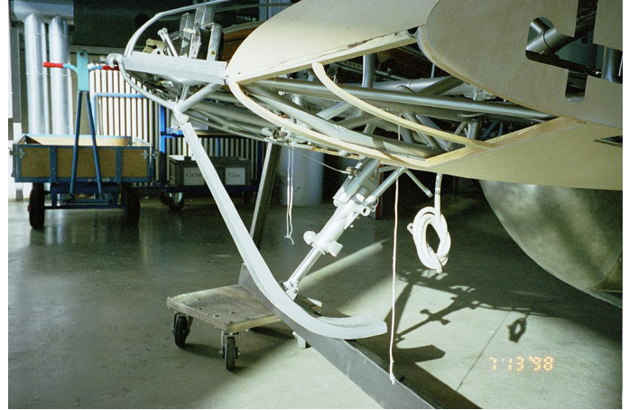
ABOVE: Horten IV nose skid that is retractable. (Photo by Russ Lee; Source: Nurflugel.com)
