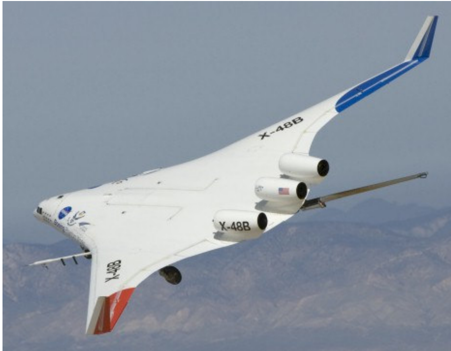
The Boeing X-48B Blended Wing Body sub-scale research aircraft banks smartly in this block 2 flight phase image, April 4, 2008. NASA Dryden Flight Research Center Photo Collection: http://www.dfrc.nasa.gov/Gallery/Photo/X-48B/Small/ED08-0092-02.jpg
