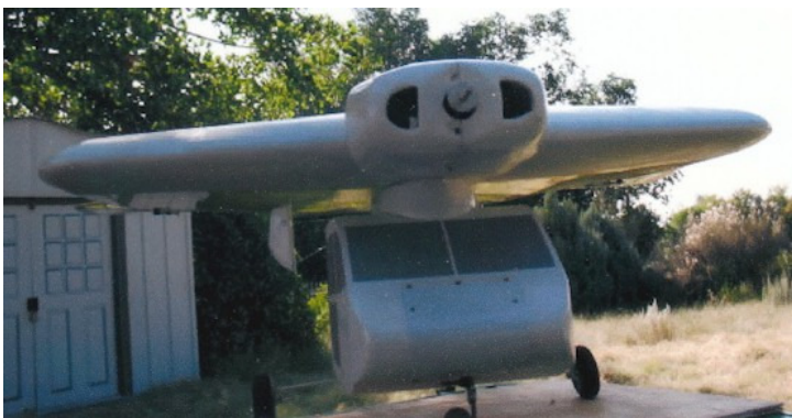
Above and below are Jim’s single strut configuration connecting the pod fuselage and wing.
