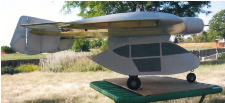
Above and below are Jim’s single strut configuration connecting the pod fuselage and wing.
