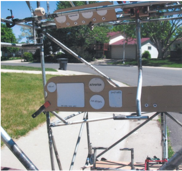
Above – Instrument panels and overhead controls. Below – Throttle-fuel mixture controls on left and elevon mixer on the right.
