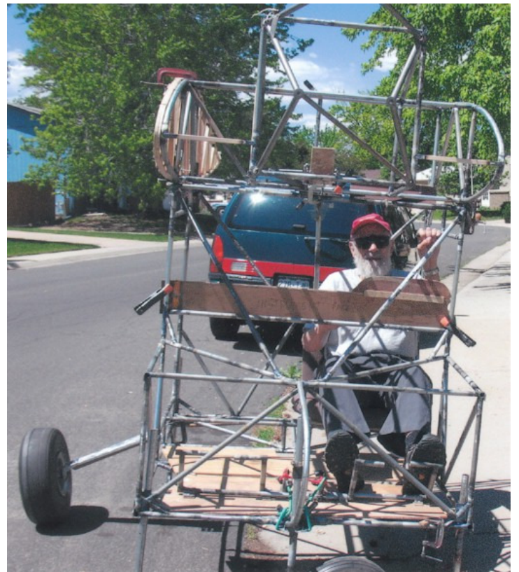
Above – Testing control placement from front.
