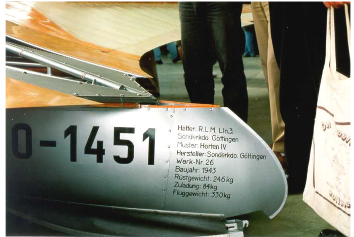
ABOVE: Bottom aft part of the Horten IV fuselage pod with all the data. The data was reconstructed by Mr. Peter Hanickel with the help of old photos. He found that there was a mistake in the book Nurflugel by Dr. Reimar Horten and Mr. P.F. Selinger. The photos are shown on page 105 of the book and the mistakes are on pages 102 & 229. The Werk-Nr. 16 is not D-10-1452, but D-10-1451.
