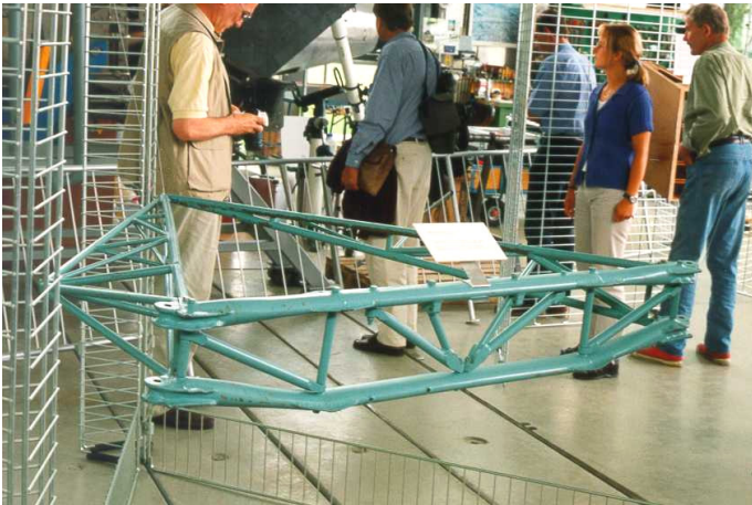
ABOVE: Remains of the center section from a Horten HoIVb. I have no details on the history of these parts. (ed. - Perhaps Russ Lee can give us a little more information on the origin of some of these parts, since I believe most of them came from the NASM for the German restoration project.)
