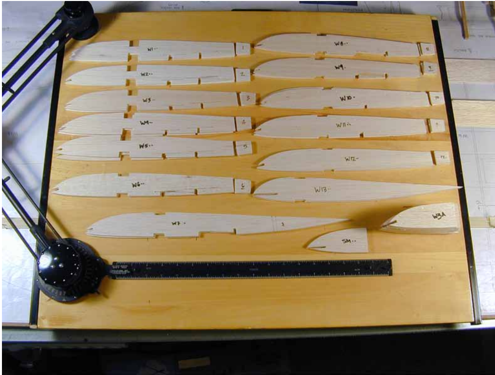
Left: All of the wing ribs cut out — 22 “standard” ribs, two for the rib separating the elevator and aileron, a shortened
