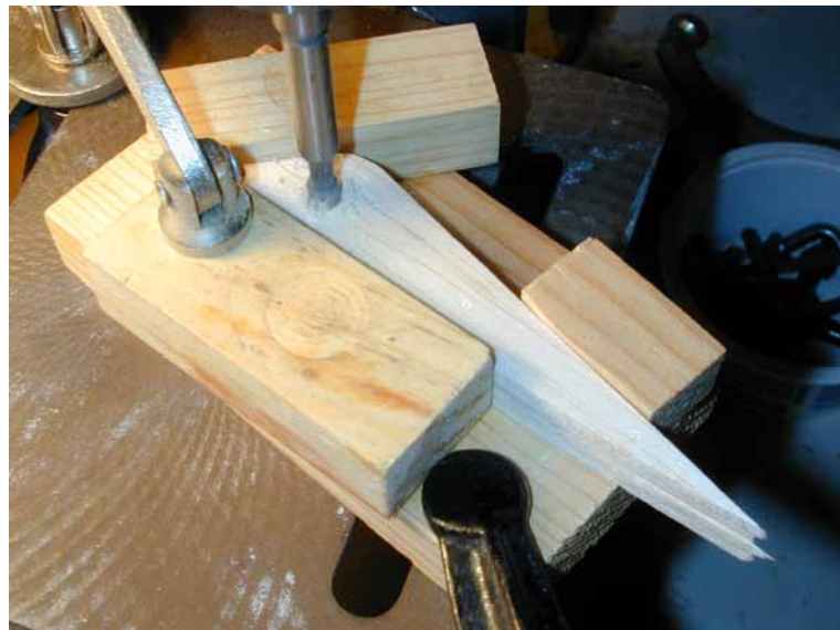
Here's the aileron rib fixture mounted on the drill press and in use. It was set up with the metal template in place so the drill bit would hit the right spot. In this shot four ribs are being drilled at the same time. The consistency was worth the extra effort.
