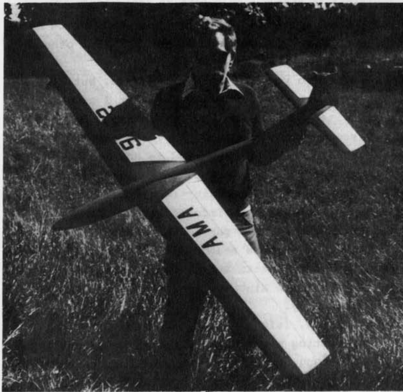
GARY WAGNER'S 2-METER SAILPLANE SEEN AT WINTONBURY, CT MEET. SHIP FEATURES BUILT-UP, FULLY-SHEETED WING WITH HUGE FLAPS AND SMALLISH AILERONS. BEAUTIFUL CRAFTSMANSHIP THROUGHOUT. FINISH IS DOPE OVER DOMESTIC TISSUE TRIM.
