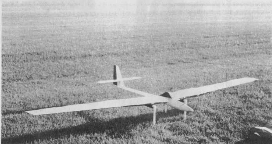
PVC PIPE SUPPORT AND REFLECTIVE COVERS OVER THE WINGS OF THE NEW MEXICAN SAILPLANE SYNERGY II.
