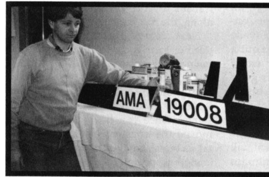
Stencils applied to wing, but prior to masking with newspaper.
