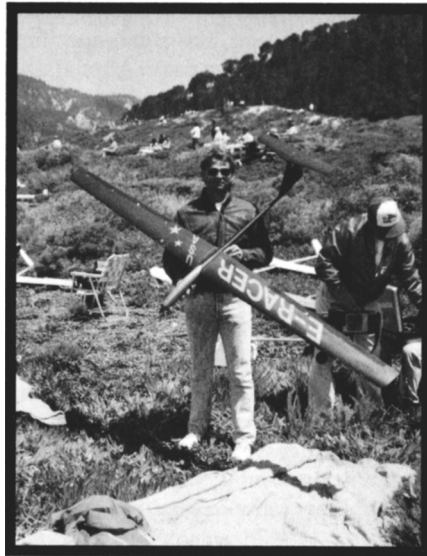
Wil Byers' E-RACER with 96" wing span and E-221 airfoil. It has a beautiful finish & great workmanship. It flew extremely well. This photo was taken by Jerry Slates at the July 7-8th Davenport Slope Race.
